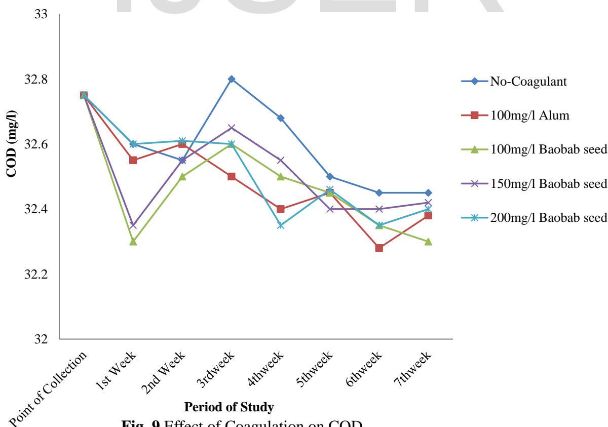
Fig. 9 Effect of Coagulation on COD
